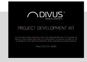
Normally, programming of DIVUS OPTIMA is performed direct- The PDK contains a virtual web server that simulates DIVUS ly on the KNX CONTROL device used. Since one does not al- OPTIMA locally on a PC. The programming and use of the visuways have such a device at hand, with the PDK it was possible alization is, except for a few restrictions, identical to a KNX CONTROL device.
